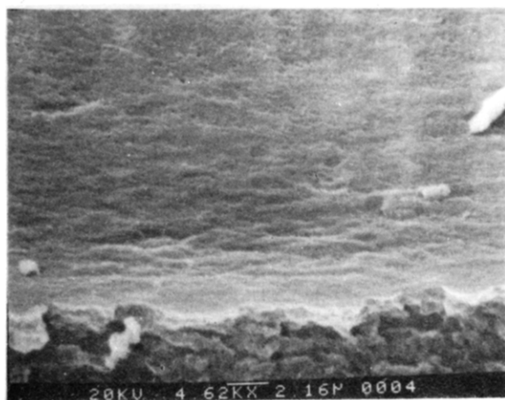
Figure 18. Scanning electron micrograph of the surface and cross section of layer in contact with the thin conducting material for a thermal-cast PMMA membrane from 15 wt % solution. Pores on the top surface are less than 0.1 \mu\text{m} in diameter. Scale bar corresponds to 2.16 \mu\text{m} .
