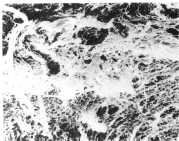
Figure 14. Scanning electron micrograph of the surface of the thermal-cast PMMA membrane in contact with the thermal insulator. The starting solution is 10 wt % PMMA, and pores on this surface are 2–15 \mu\text{m} in diameter. Scale bar corresponds to 13.7 \mu\text{m} .
